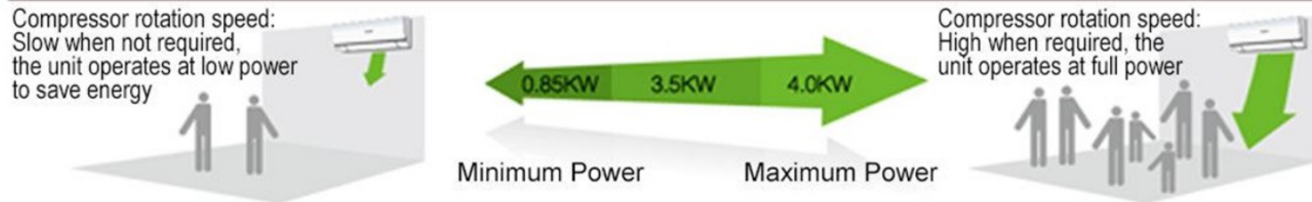
Graph shows the 1.5HP Inverter model's wide power output range during cooling
